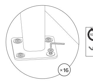
Fully tighten bolts once all legs are aligned on table top.
