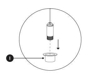
Unscrew socket ring (I) from socket before attaching shade.
