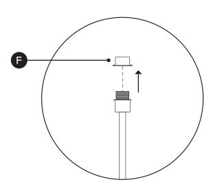
Unscrew socket ring (F) from socket before attaching shade.
