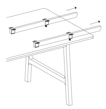
Unscrew levelers slightly to release extension support bars.
