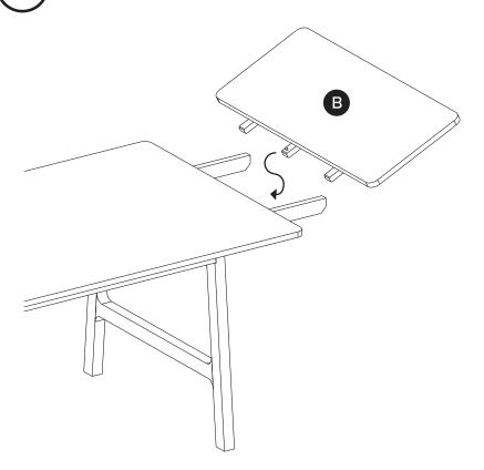
Ensure that metal peg fits into hole on underside of table top.
