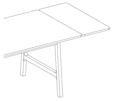
Tighten levelers to secure and align leaves with table top.
