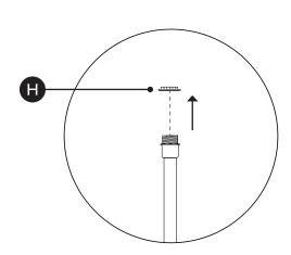
Unscrew socket ring (H) from socket before attaching shade.
