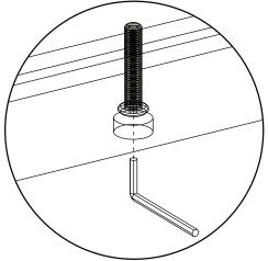
If bolts are too loose: arms can extend too far and come out of the table completely. If bolts are too tight: arms will not extend far enough to align with dowels on leaf.
