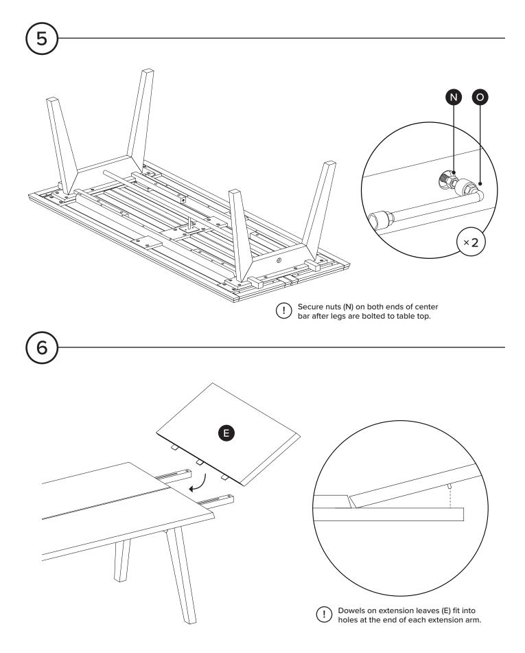
If the dowels on one or both of your extension leaves don't fit properly into the extension arms, the bolts on the arms underneath the table top need to be adjusted. Loosen the bolts to move the arms farther out from the table, and tighten to move the arms farther inward.
