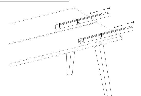
Start with adjusting the bolt on the back of the arm:
