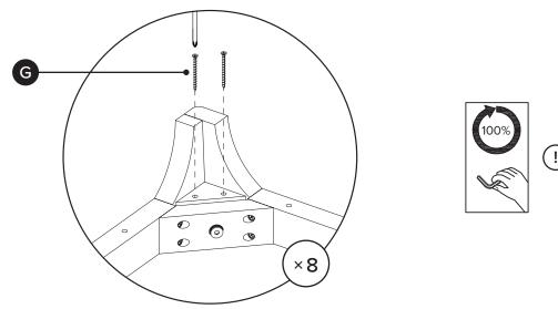
Fully tighten all bolts (E) and screws (G) once legs are aligned properly.
