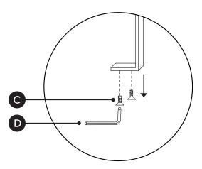
Unscrew bolts (C) from lamp stand (A) before attaching lamp stand to base (B).
