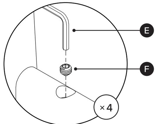
! Fully tighten all screws (F) once legs are attached to table top.
