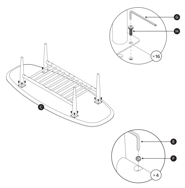
Fully tighten all screws (F) once legs are attached to table top.
