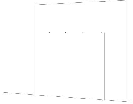
Locate wood wall studs and mark screw placement on wall 16" apart where cleats (B) should be mounted.
