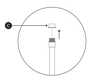
Unscrew socket ring (C) from socket before attaching shade.
