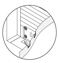
Place the wheels at the bottom of the door into the outer groove.
