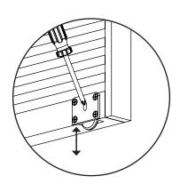
Adjust the wheel at the bottom of doors by screwing in or out if the door is not straight.
