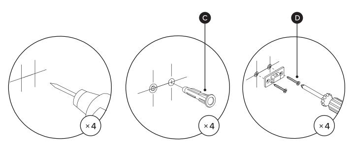
Drill holes in wall using 8mm / 5/16" drill bit.
