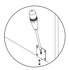
Adjusting the wheel at the bottom of door by screwing in or out when the door does not fit to assemble or it's loose after assembling.
