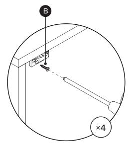
Attach pair of brackets to top corners of the back unit.
