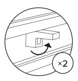
Unlock mechanism underneath table edges first. Two people should pull table sections apart.
