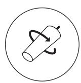
Secure all four legs into pre-drilled holes as shown in the diagram above by rotating the legs clockwise until fully tightened.
