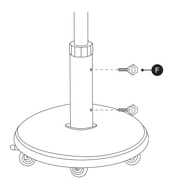
Fully tighten both screws (F) to stabilize umbrella in base.
