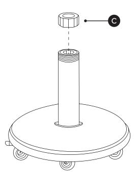
Do not fully tighten cap (E) before inserting umbrella.
