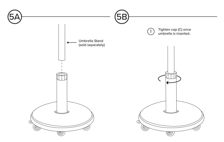
After the casters (G) are installed and patio umbrella are properly inserted, make sure all four casters (G) are locked by pressing down the wheel brake to secure. To unlock it, simply pull the leverage back up to move your umbrella base.
