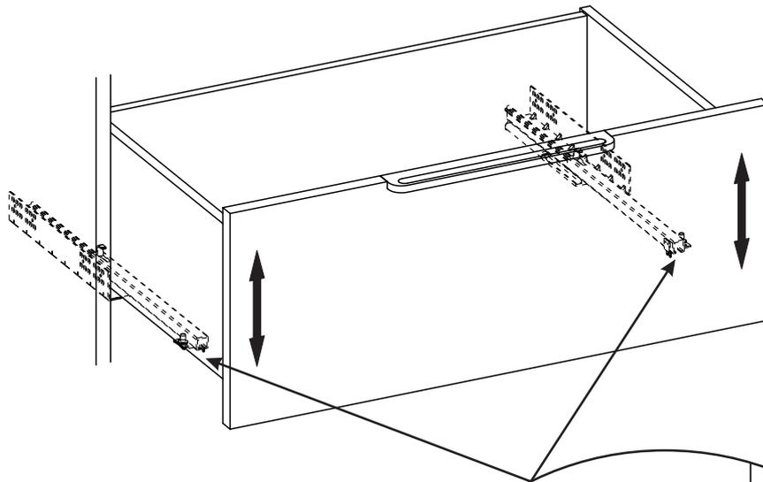
ⓘ Adjust levers on either side of drawer as needed to straighten drawer.
