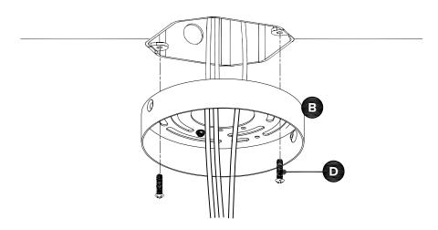
Thread wires through mounting bracket iron round (B) before attaching to junction box.
