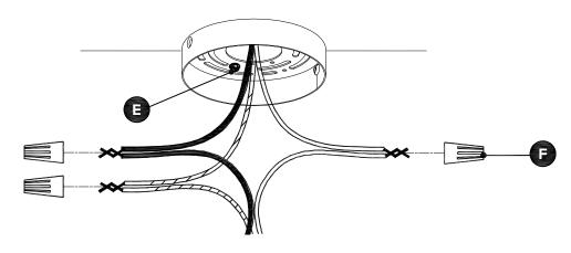
If junction box does not have a green ground wire, attach ground wire from lamp to short green screw (E) on mountingbracket.
