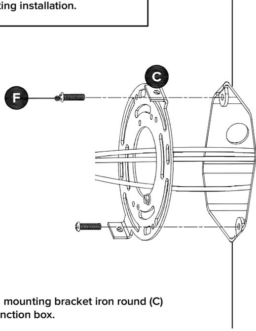
Thread wires through mounting bracket iron round (C) before attaching to junction box.
