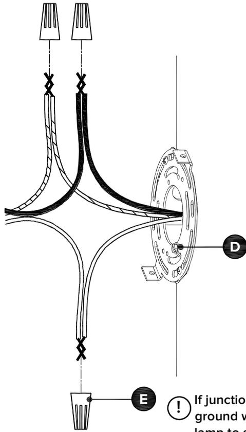
If junction box does not have a green ground wire, attach ground wire from lamp to short green screw (D) on mountingbracket.
