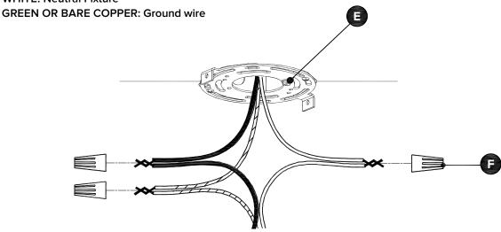
If junction box does not have a green ground wire, attach ground wire from lamp to short green screw (E) on mountingbracket.
