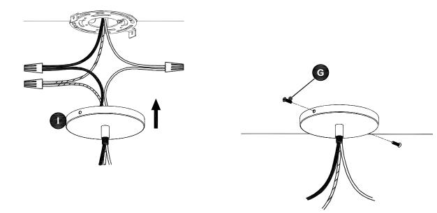
Align one side first then tighten 50% then align other side and fully tighten.
