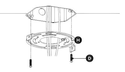
Thread wires through mounting bracket iron round (H) before attaching to junction box.
