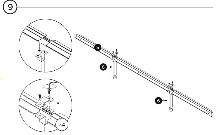
Attach floating center legs where labels are situated on center beam (5). Ensure that legs are straight, perpendicular to center beam.
