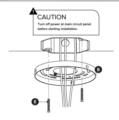
Thread wires through mounting bracket iron round (B) before attaching to junction box.
