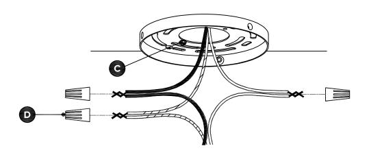
If junction box does not have a green ground wire, attach ground wire from lamp to short green screw (C) on mountingbracket.
