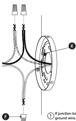
If junction box does not have a green ground wire, attach ground wire from lamp to short green screw (E) on mountingbracket.
