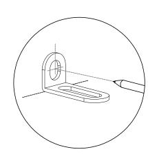
Place unit in desired location and mark on wall where holes should be drilled.
