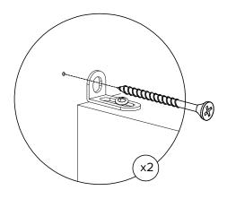
Drill holes into drywall, and attach unit to wall with appropriate hardware.
