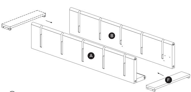
(!) Assembly tip : align (A) and (B) at its position properly by using part (F).
