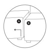
To separate sections, lift section with pegs straight up and out of the teeth of the clips.
