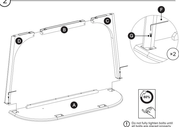
Do not fully tighten bolts until all bolts are placed properly
