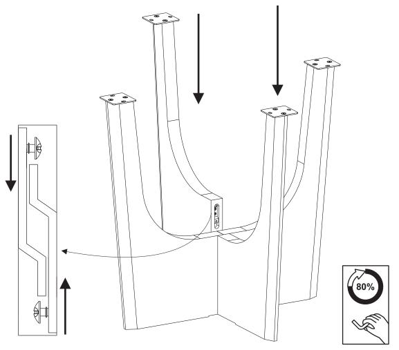
Do not fully tighten bolts until all bolts are placed properly
