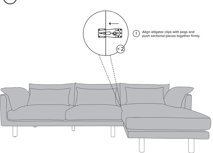
To separate sections, lift section with pegs straight up and out of the teeth of the clips.
