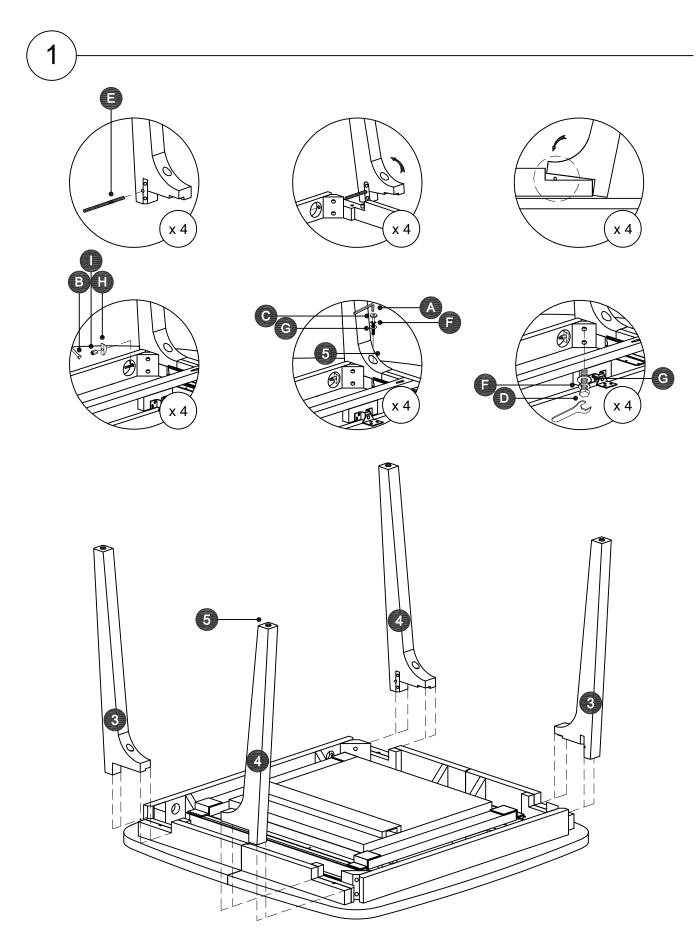
Noted: Adjust the leg aligned with apron before tighten all bolt
