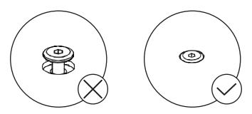
! Once all bolts are placed, completely tighten
