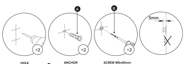
HOLE Drill hole in wall with drill bit 8mm
