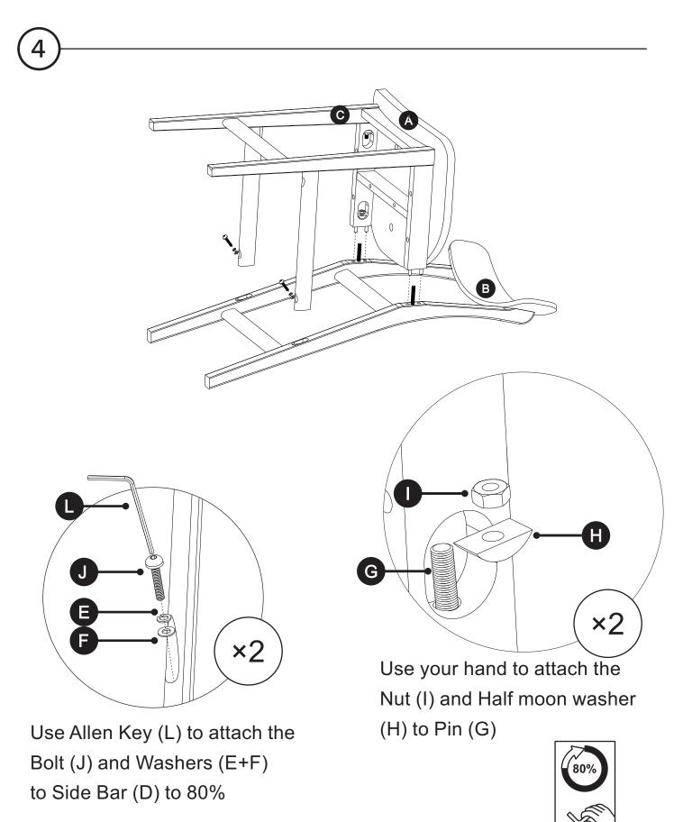
Tighten all Bolts (J) with Allen Key (L) and Nut (I) with Spanner (K) to 80%
