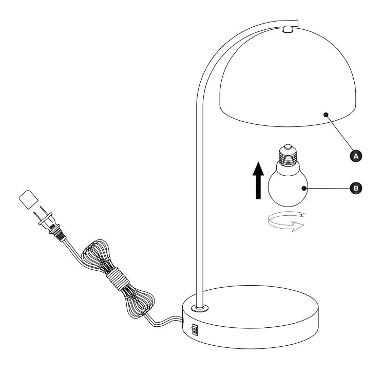
Remove plug out the power socket during bulb attachment.
