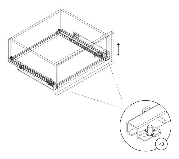
Adjust levelers on either side of drawer as needed to straighten drawer.
