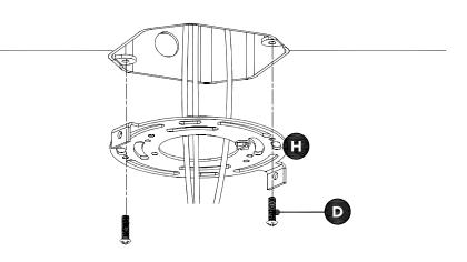
Thread wires through mounting bracket iron round (H) before attaching to junction box.
