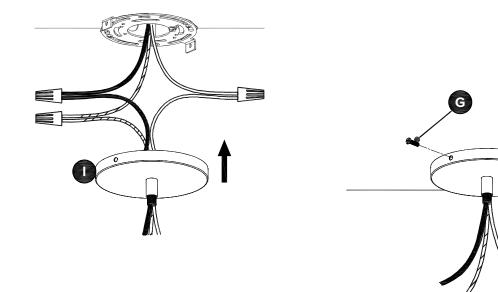
Align one side first then tighten 50% then align other side and fully tighten.
