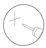
Drill hole in the wall using the drill bit.
