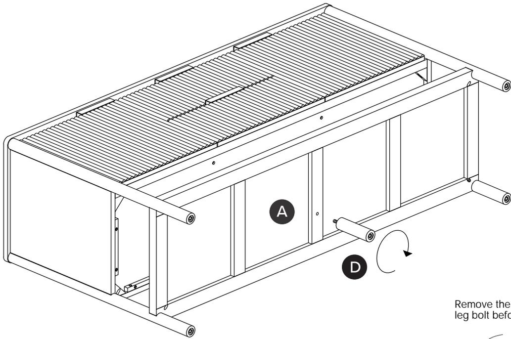
Remove the protection on the leg bolt before assembling
