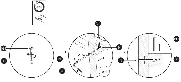
Note: use bolt (N1) as a tool to insert temporarily and hold nut (P) to holes underneath the seat, while connecting bolt (N) to nut (P).
