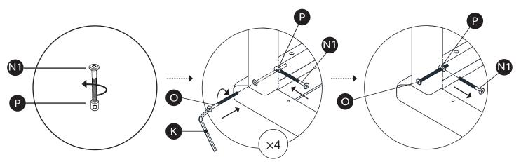
Note: use bolt (N1) as a tool to insert temporarily and hold nut (P) to holes underneath the seat, while connecting bolt (O) to nut (P).
