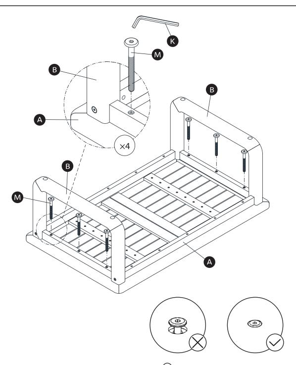
(!) Once all bolts are placed, completely tighten all bolts
