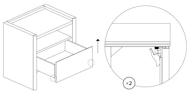
Turn the orange adjustment wheel on the drawer glides in the direction of the arrow.
