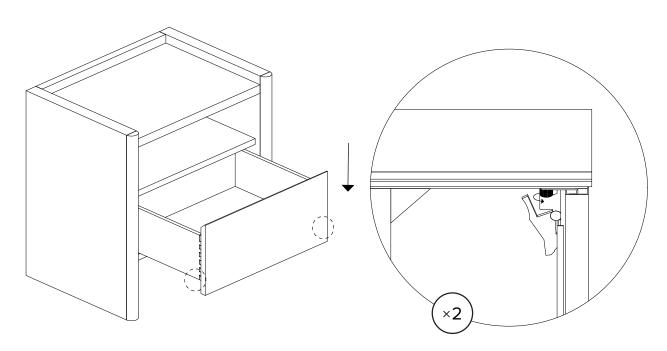
! Turn the orange adjustment wheel on the drawer glides in the direction of the arrow.
