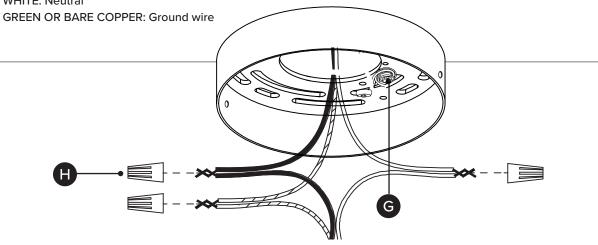
If junction box does not have a green ground wire, attach ground wire from lamp to short green screw (G) on mounting bracket.
