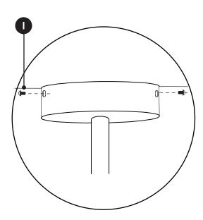
Align the canopy hole to the mounting bracket to screw them together.
