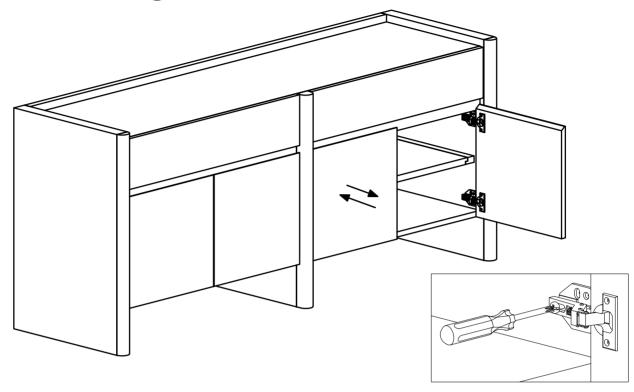
If the door is crooked, adjust hinge(s) up or down:
