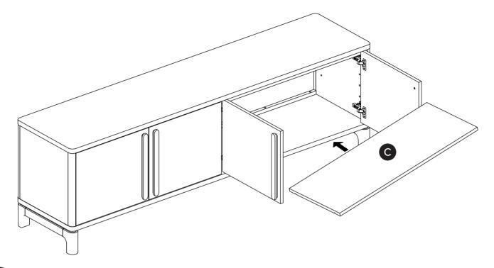
Lift the shelf C upwards when attaching the shelf pin H at the choosen location
