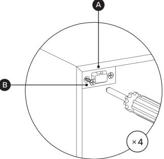
Attach pair of brackets to top corners of the back of the unit. Note there are no existing pilot holes on the product.
