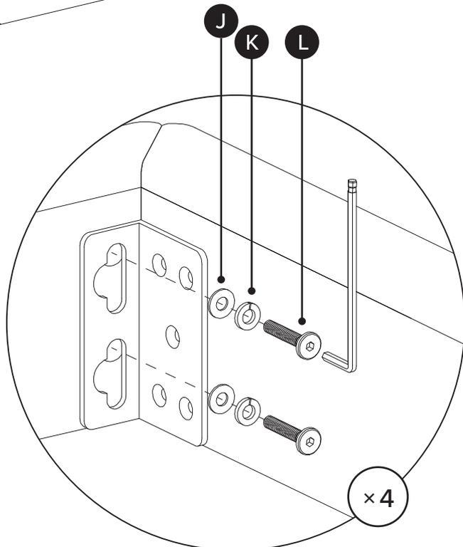
! Turn the bolt (L) by hand first. Fully tighten bolts (L) on corner frames after the side rails are flat.
