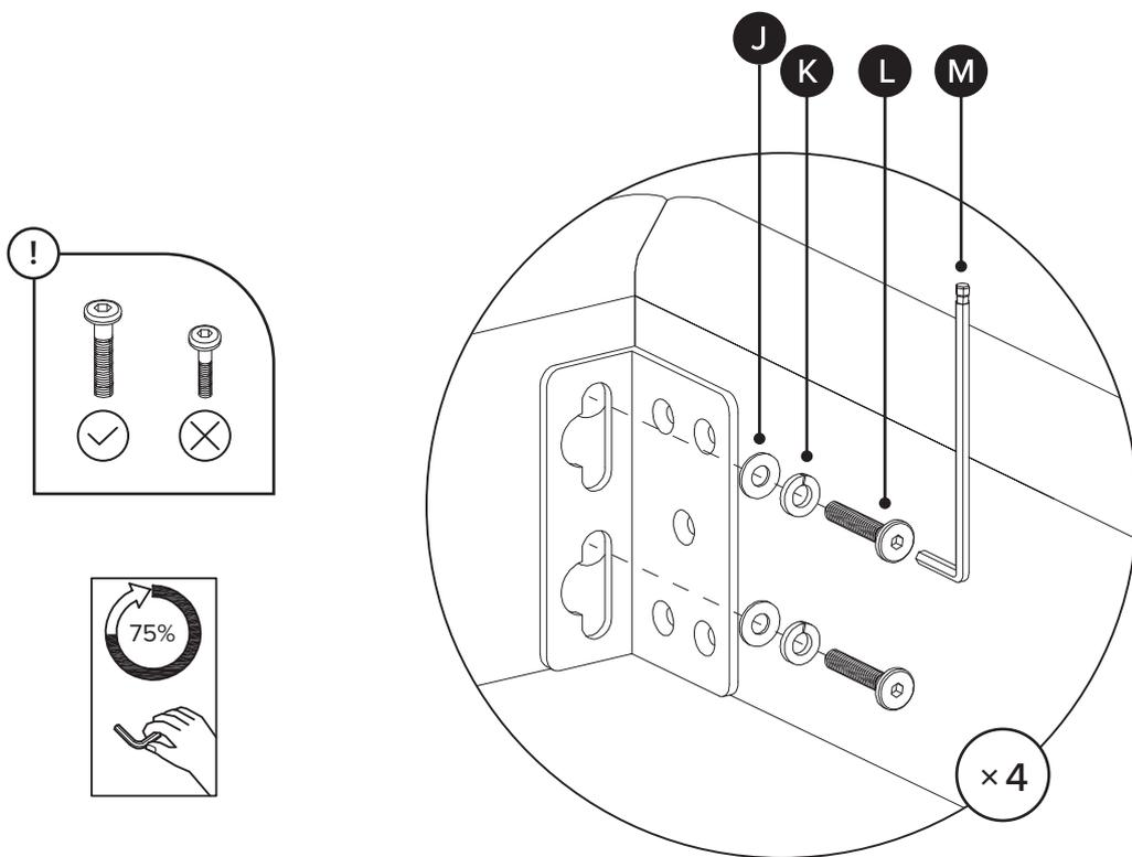
! Turn bolts (L) by hand first. Do not fully tighten bolts (L) on corner frames until step 2.
