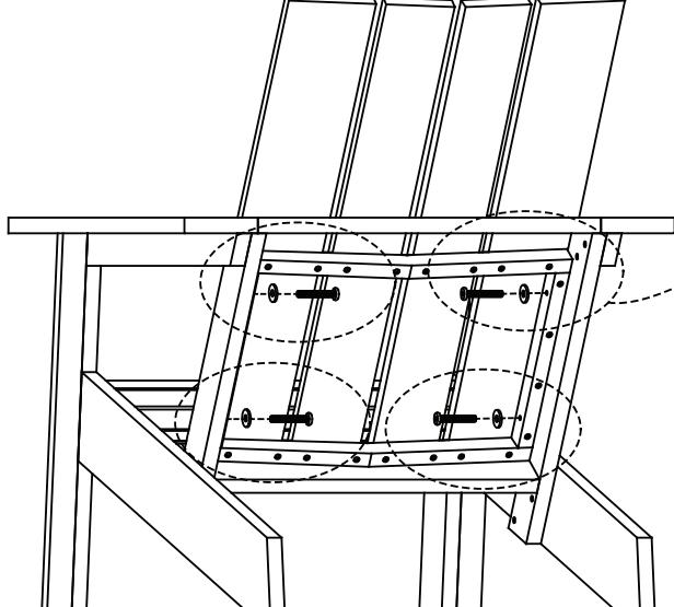
! Step 2: Once all bolts are placed, completely tighten all bolts.
