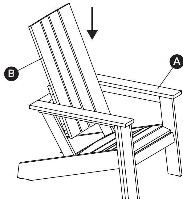
! Step 1: Do not completely tighten bolts.
