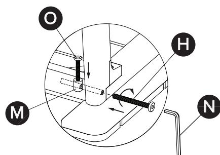
Bulong (H) has to turn toward the right direction to connect with nut (M).
