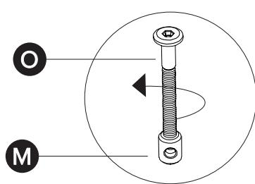
! Note: Use bolt (O) as a tool to insert temporarily and hold nut (M) to holes underneath the table, while connecting bolt (H) to nut (M).
