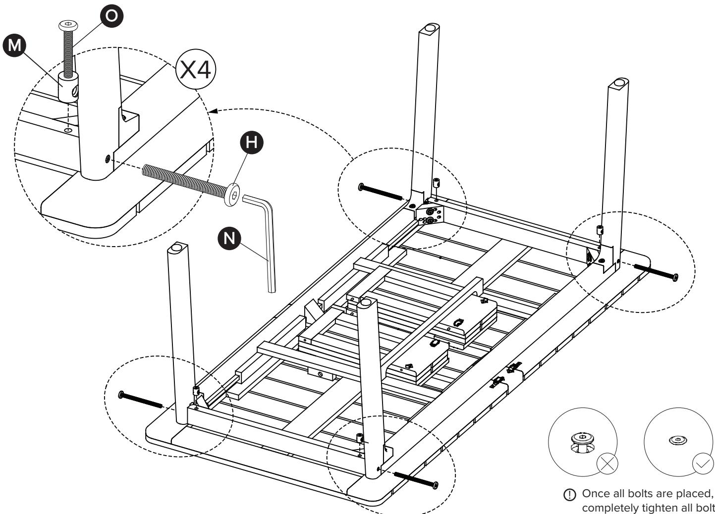
! Once all bolts are placed, completely tighten all bolts
