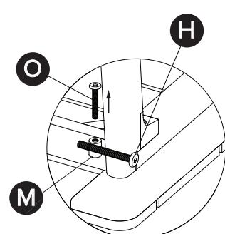
Remove bolt (O) after nut (M) is completely attached to bolts (H).
