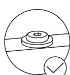
! Step 2: Once all bolts are placed, completely tighten all bolts.
