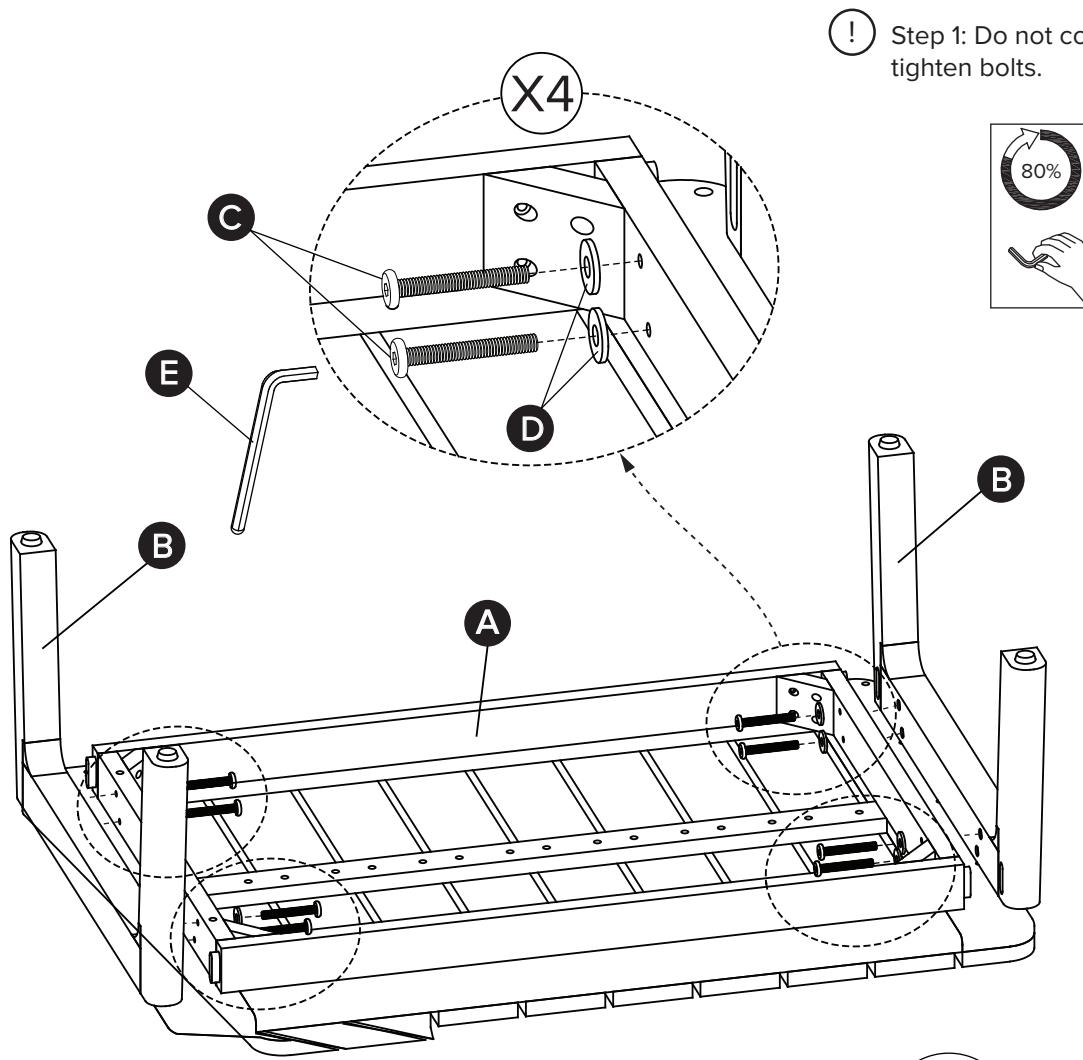
! Step 1: Do not completely tighten bolts.
