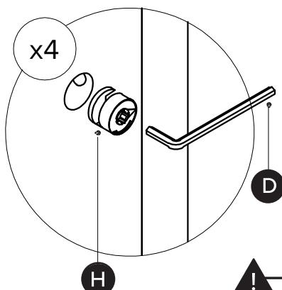
! Tighten 100% by rotating part (H) 90 degree.
