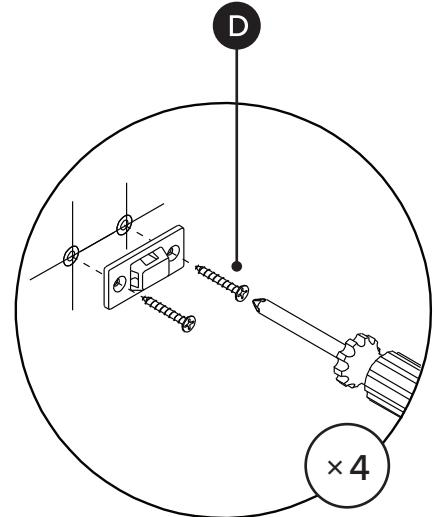
Drill holes in wall using 10mm / 13/32" drill bit.
